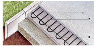
1 = béton 2 = tapis chauffant 3 = support
