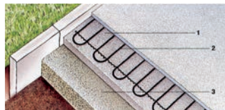
1 = béton 2 = tapis chauffant 3 = support
