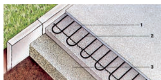
1 = béton 2 = tapis chauffant 3 = support
